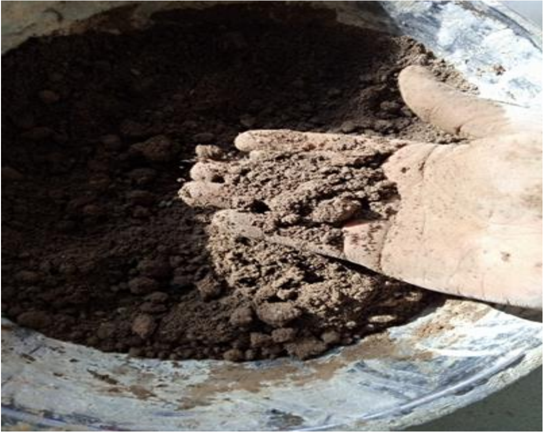
Plate 3.5: Break down of lumps more than 200mm in diameter
