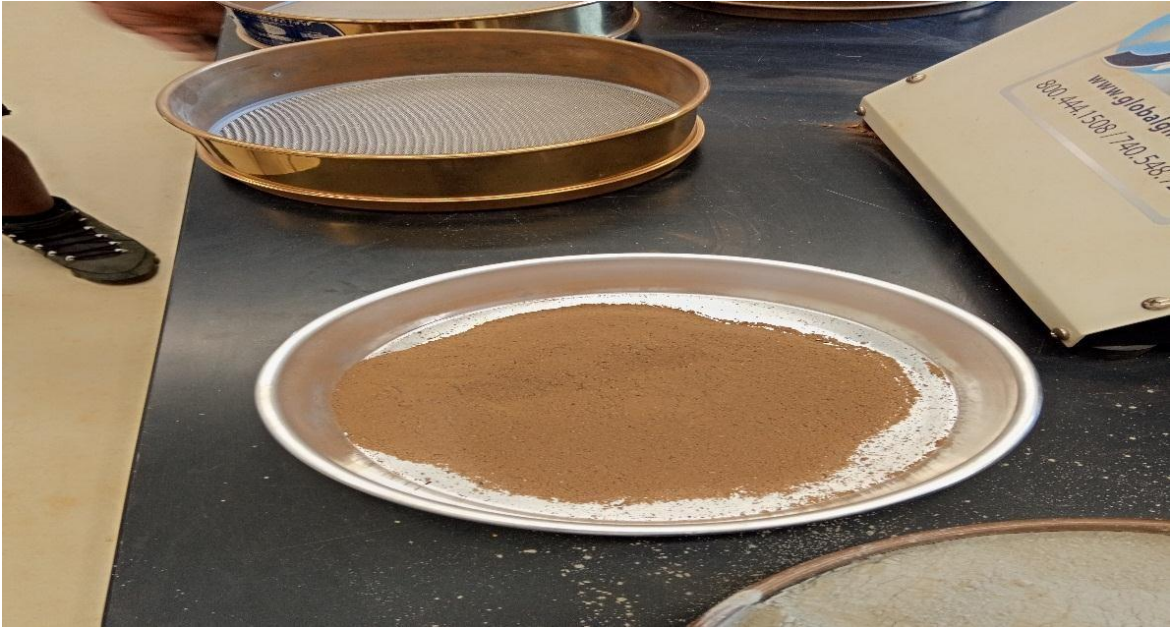
Plate 3.3: Sample of Palm Kernel Shell Ash Used
