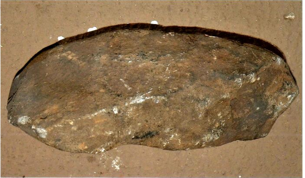
Plate 4.2a: A piece of Basalt (The crystals are not visible to the naked eyes).
