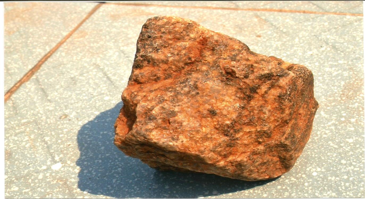
Plate 4.1a: A piece of Granite rock (The large crystals are visible to the naked eyes).
