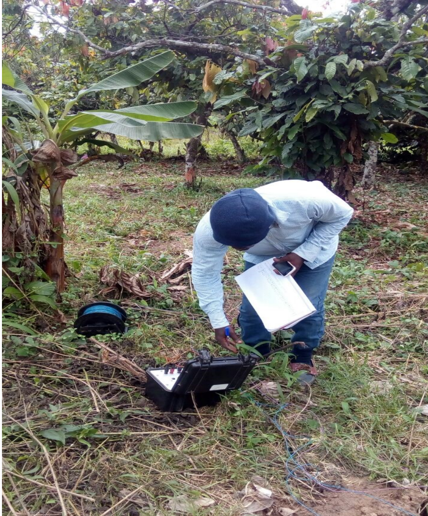
Figure 3.2: Electrical earth resistance measurement taken with allied Omega resistivity meter.
