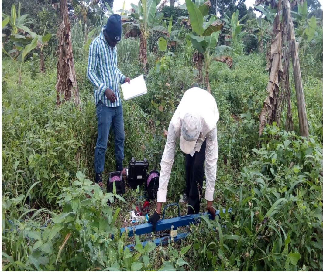
Figure 3.1: Electrical earth resistance measurement taken with resistivity meter using electrodes mounted in a fixed configuration at kola farm
