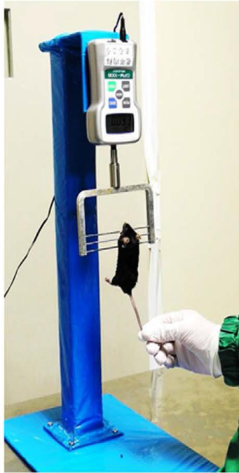
Figure 2.22 Forelimb Grip Strength Test (Smith, et al. , 1995).
