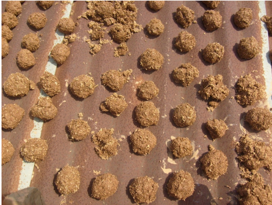
Plate 2.4: Rice husk made into cake balls before incineration
