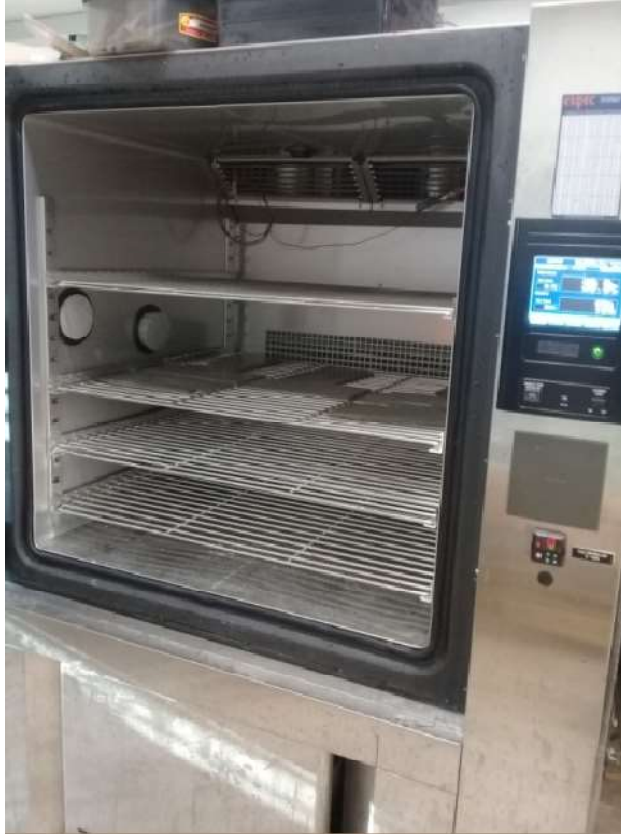
Plate 3.9: Dry accelerated carbonation of composites
