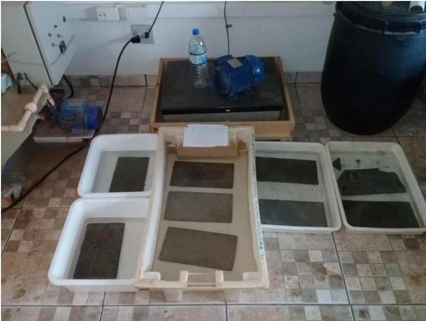
Plate 3.11: Soaking of accelerated carbonated samples in water for thermal curing
