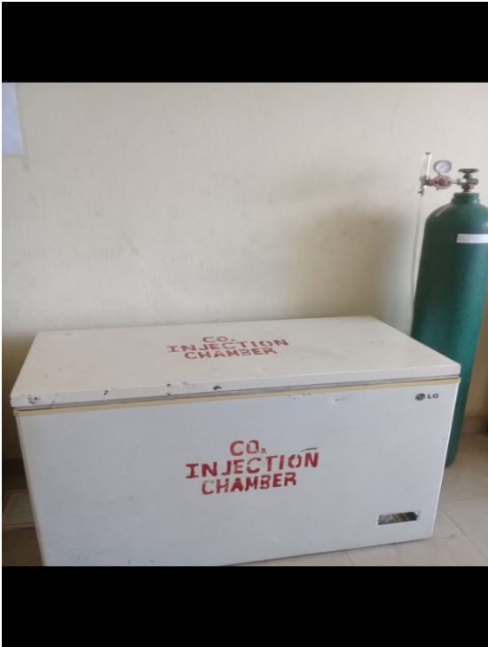
Plate 3.7: Wet carbonation of composite samples
