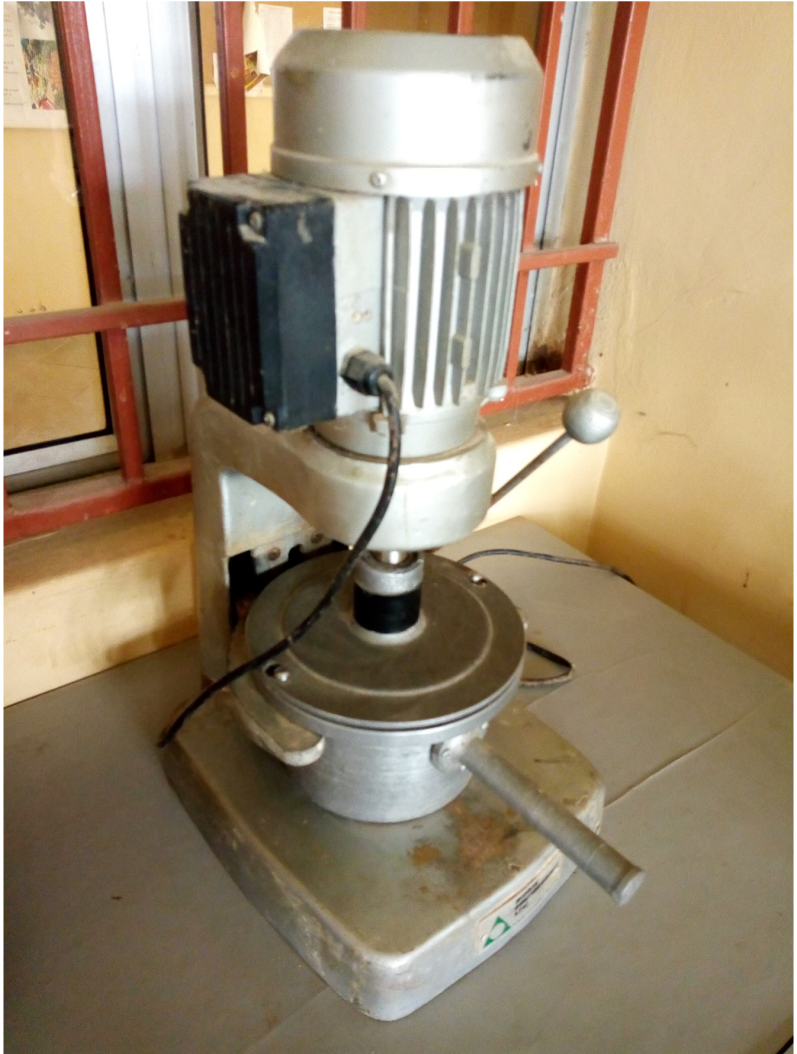
Plate 3.3: Adapted amala preparation machine
