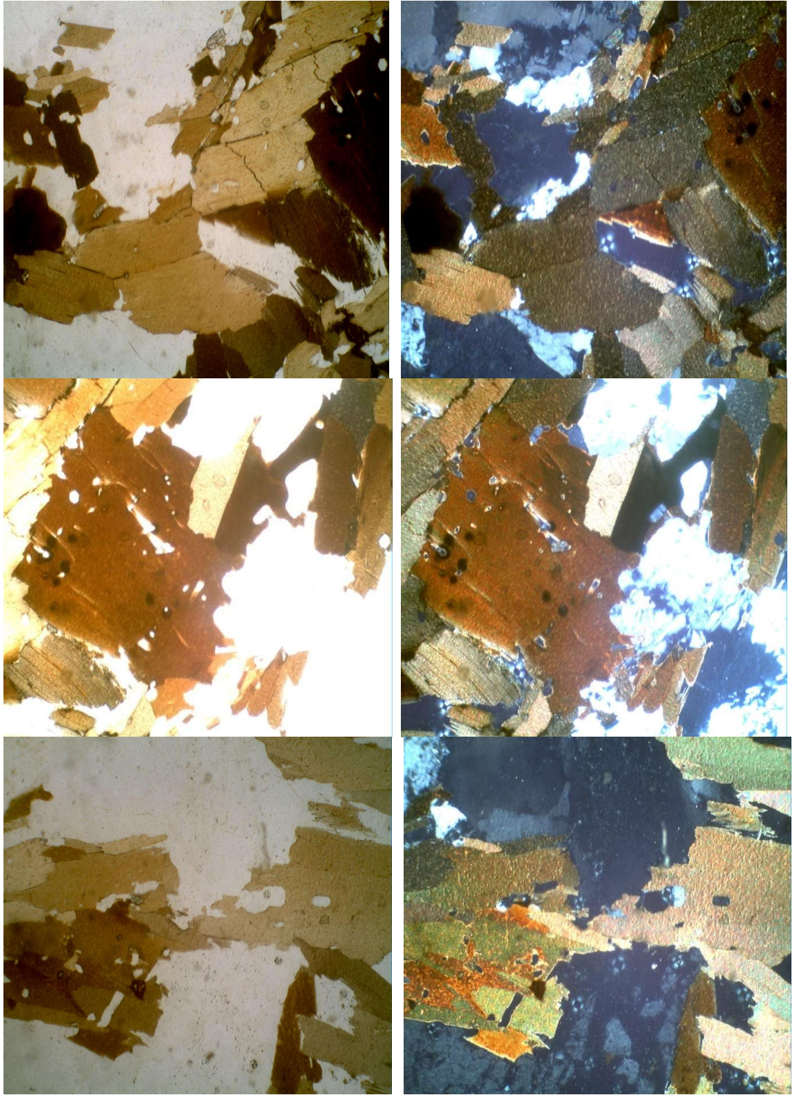
Fig. 4.23:Photomicrograph of granite of Wonu, Ibadan-Apomu area showing quartz, plagioclase feldspar, microcline, biotite, muscovite, hornblende and augite.
