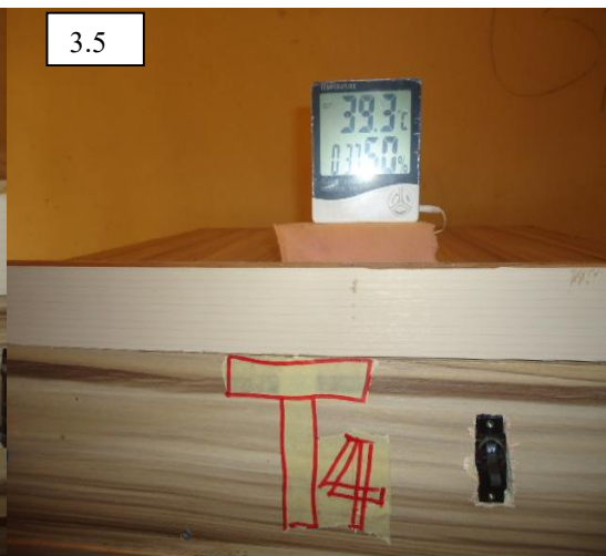
Plate 3.5: Fabricated incubator calibrated at 39°C representing High incubation temperature
