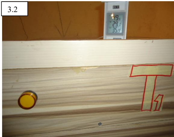
Plate 3.2: Fabricated incubator calibrated at 36°C representing Very low incubation temperature
