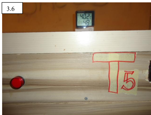
Plate 3.6: Fabricated incubator calibrated at 40°C representing Very high incubation temperature
