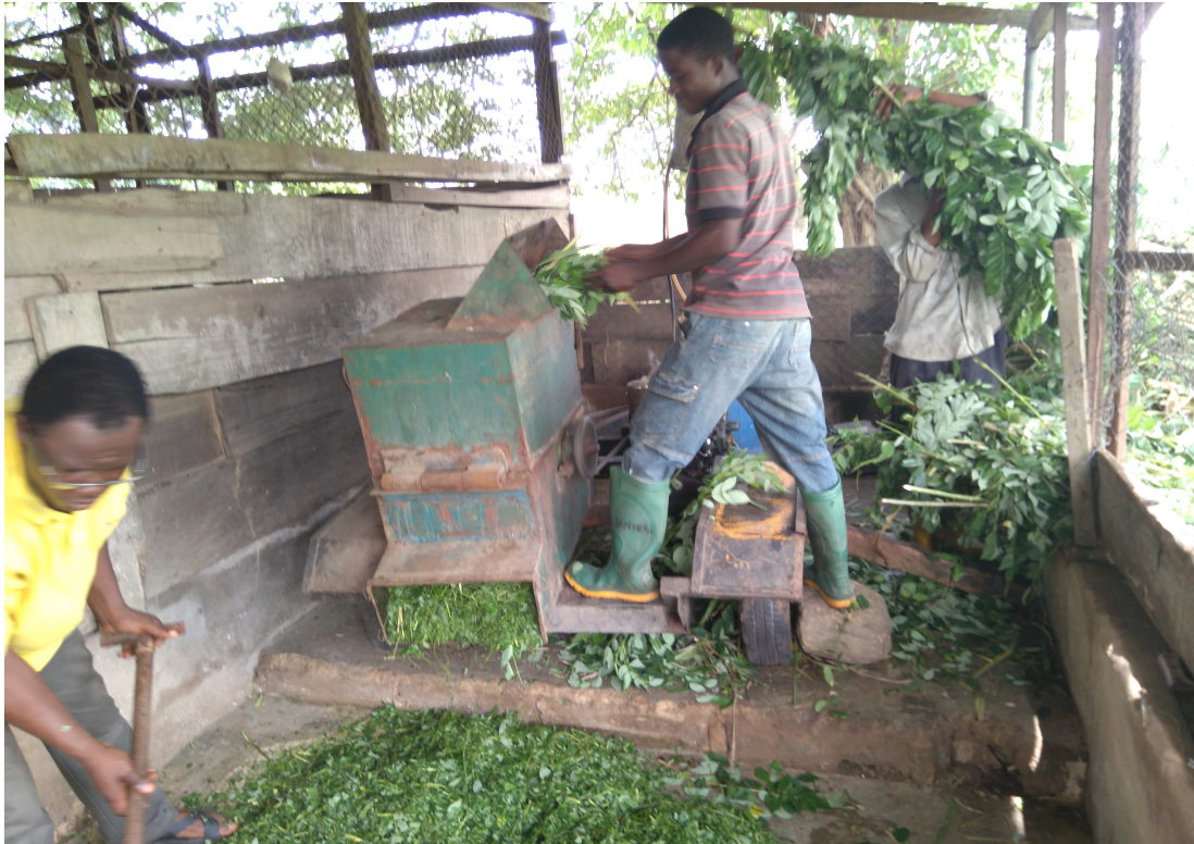
Plate 4: Particle size reduction of Forages with a Mechanical Chopper
