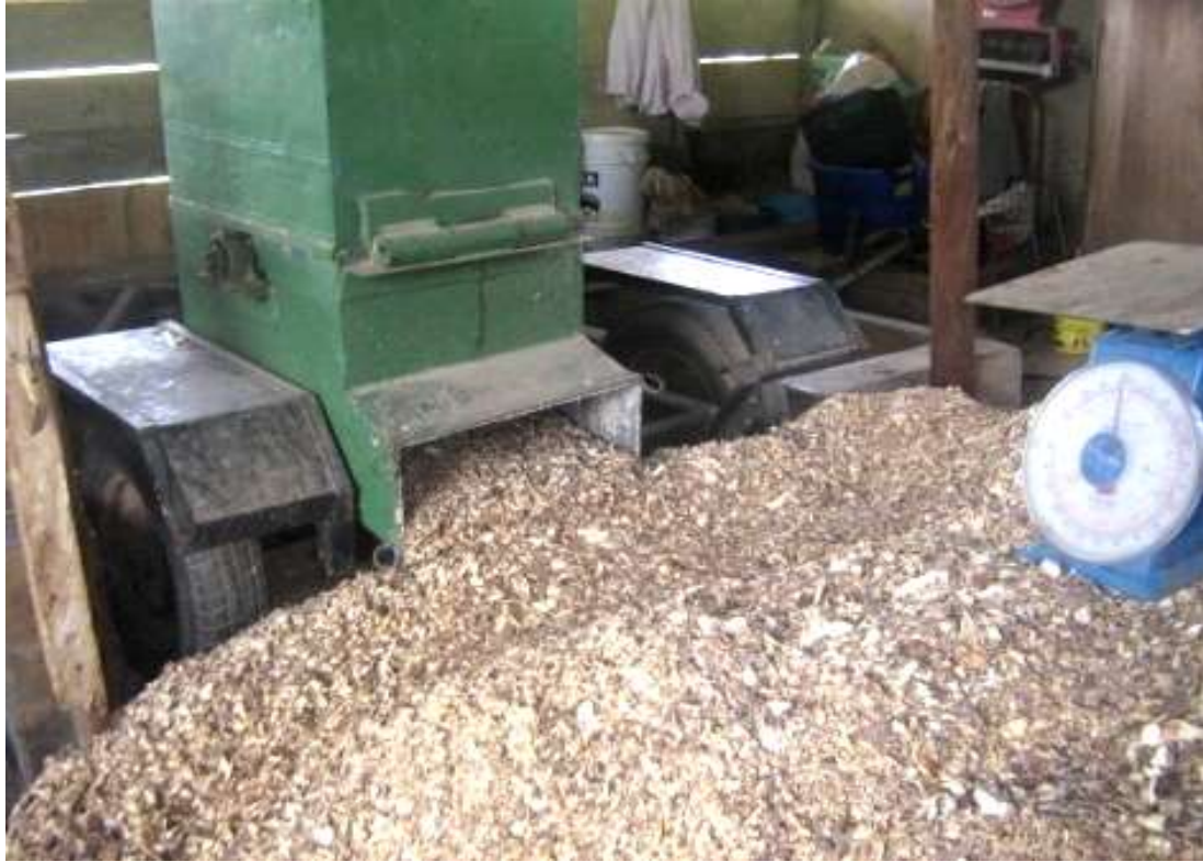
Plate 5: Particle size reduction of cassava peels with a Mechanical Chopper
