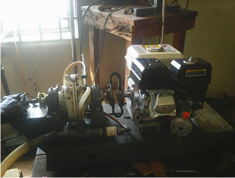
(a) Coupling of engine to Dynamometer
