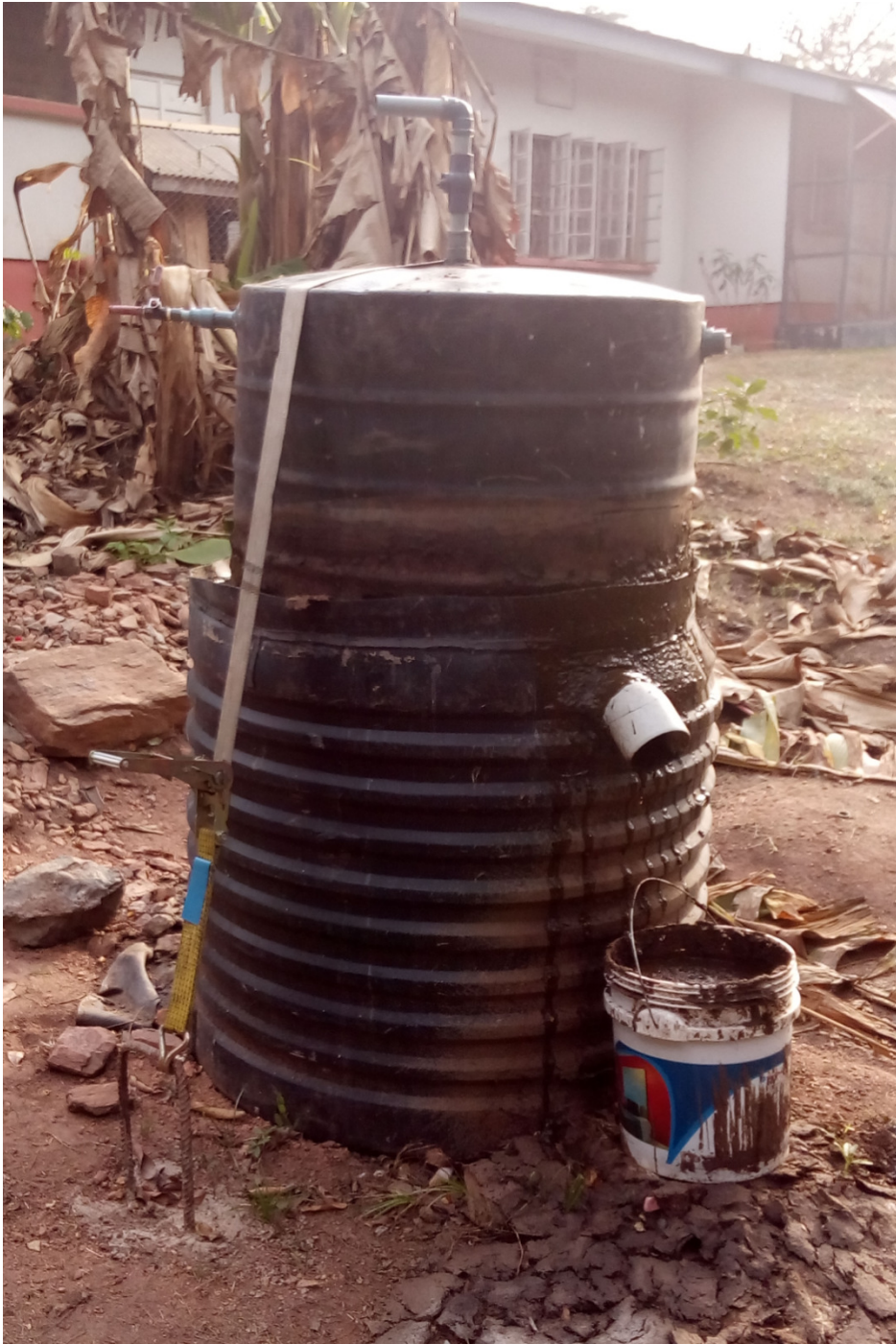
Improvement of digester with clamps and belt to hold gas cap in place
