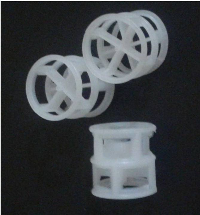
Plate 3.2: Pall Rings used as Packing Material in the Water Scrubber
