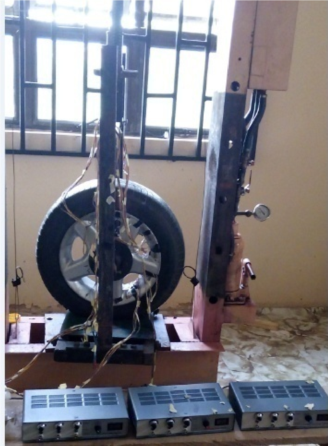
PlateC4: Wheel-tyre assembly in the test rig showing the instrument (strain measuring device) connection to the lead wires of the strain rosette.
