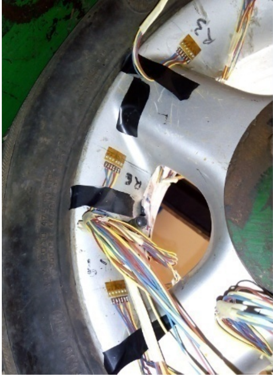
Plate C2: Wheel-tyre assembly in the test rig showing attached strain rosette at the outside surface of the rim: Outboard view.
