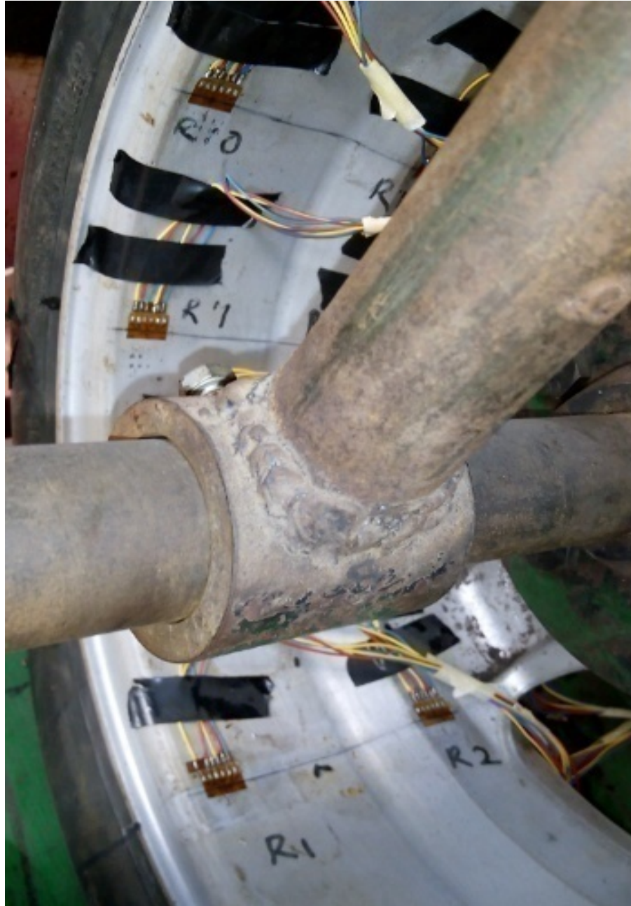
PlateC1: Wheel-tyre assembly in the test rig showing attached strain rosette at the outside surface of the rim: Inboard view
