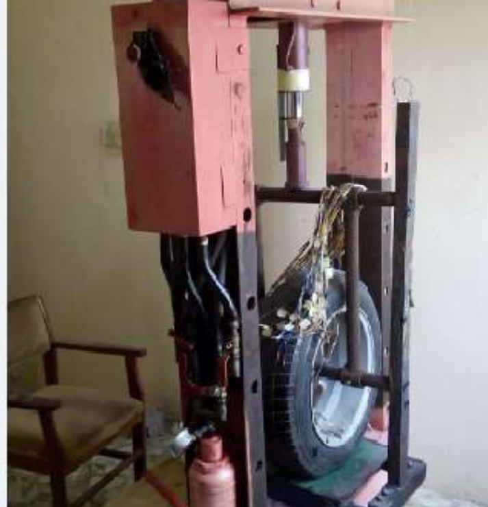
PlateC3: Wheel-tyre assembly in the test rig with lead wires.
